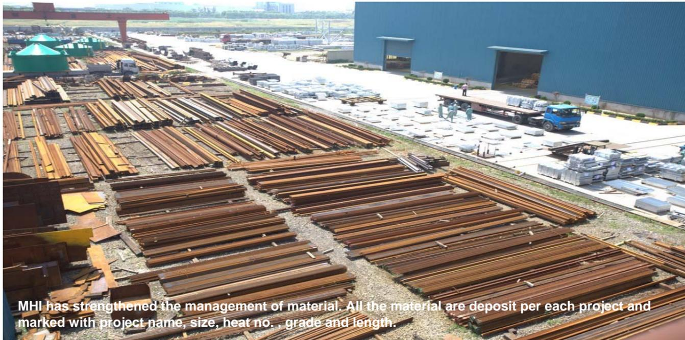
MHI has strengthened the management of material. All the material are deposit per each project and marked with project name, size, heat no., grade and length.
