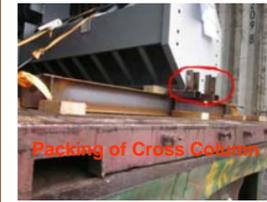
Recently, MHI is helping one of it's competitor to do the steel structure fabrication for VALE conveyor project. Attached pictures are the lifting and packing of cross column. The cross column is 6-8 tons for each, with a size of 12m (L) x 2.5m (W) x 2.5m(H).
